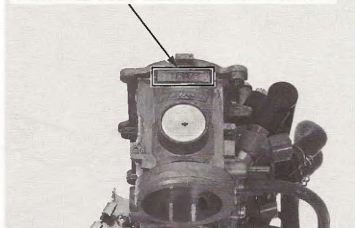
THROTTLE BODY IDENTIFICATION NUMBER
