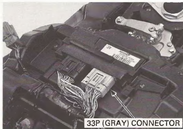
33P (GRAY) CONNECTOR (Wire side/female terminals)
