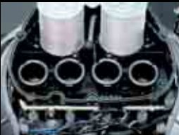
Dual Sequential Fuel Injection System - Two sets of injectors, one set high in the air box, the other at the intakes, ensures blistering response and performance across the rev range, and with a new ECU, an even smoother throttle response is achieved.
