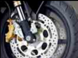
Disc Brakes - High-performance 4-piston calliper front disc brakes stop wide, floating rotors for sure, responsive braking control.
