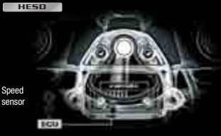
Honda Electric Steering Damper - With its advanced electro-hydraulic system pioneered and developed on the RC211V, automatically adjusts to provide unrivalled control at high speeds and light, responsive handling particularly at low speed.
